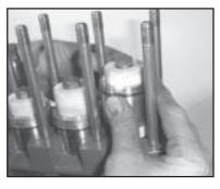
11. Press seal sleeve assembly into the manifold and seat firmly. Put the support ring (41) on plunger with v-side facing the manifold.
